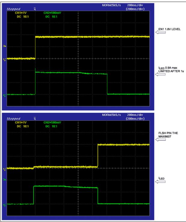
Figure 2. When EN1 goes high, the timeout period of the reset circuit is initiated and when timeout occurs it reduces the LED current by bringing its reset output high (top). When the Flash pin on the MAX8607 goes high, current to the LED is reduced, thus preventing overheating (bottom).
