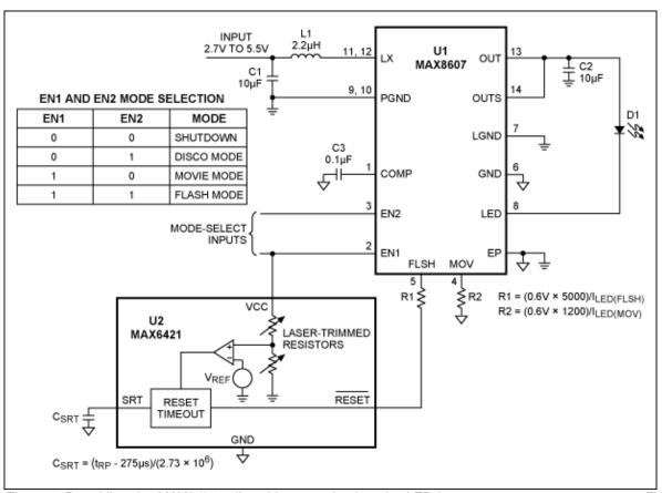
Figure 1. By adding the MAX6421 adjustable reset circuit to the LED boost converter, you can prevent Flash LED overheating and extend LED life.
